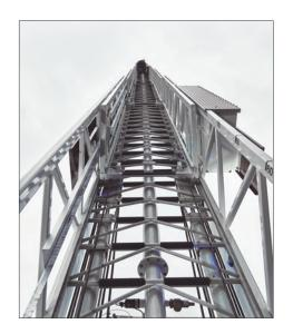
**RETRACTION OVERRIDE:** Retraction automatically stops as the the steps on the fly section near overlapping with the next lower section; this ensures crew safety and prevents potential injury. Available on Smeal aerials.
