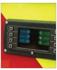
**SPARTAN SELF-LEVELING SYSTEM (SSL):**After the outriggers are deployed, the truck can be automatically leveled with a push of a button. The optional SSL system also stows the outriggers at the touch of a button. Available on Smeal aerials.
