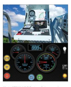
**AL-11 AERIAL LOGIC:** A totally integrated system that provides instant feedback on a ladder's extension, location, retraction, angle, load and breathing air system status, as well as J1939 engine information. Available on Smeal aerials.
