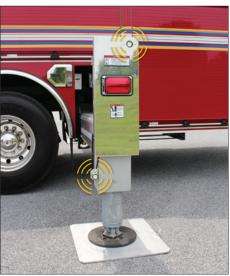
**OUTRIGGER DETECTION SYSTEM:**Automatically detects obstacles at scene to ensure secure placement of outriggers.
