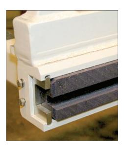
**LADDER SLIDE PADS:** Load Transfer Pads and Front, Rear, and Side Slide Pads reduce friction and ensure smooth ladder operation. Slide pads are also designed with accessibility in mind for easy inspection and replacement. Available on all models of aerials.
