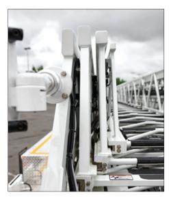
**LOWER TRAVEL HEIGHT:** Ladders stack efficiently, providing a low profile and lower travel heights, making it easy to fit into historic firehouses and under bridges. Available on Ladder Tower aerials.
